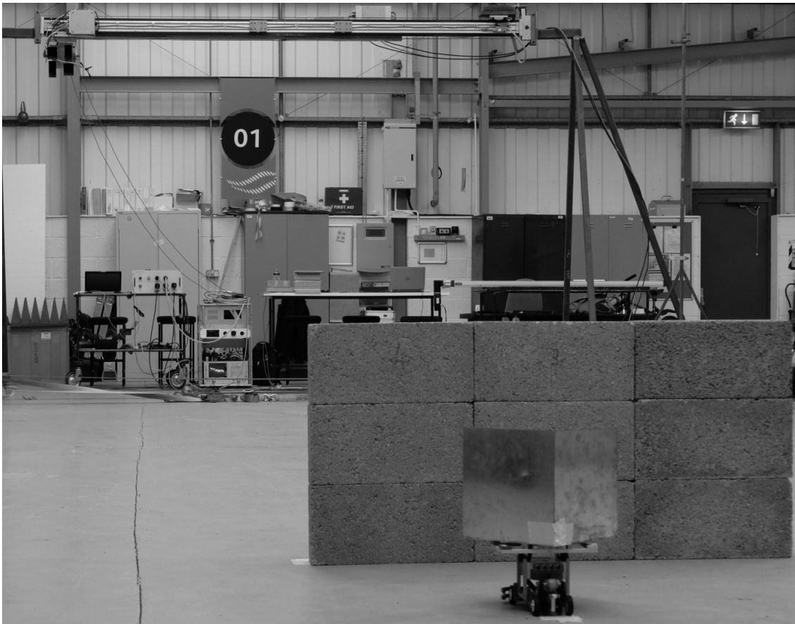
Figure 5: Experimental measurement scene set up. The 876 × 645 [mm] breeze block wall is situated 10 [m] down range from the radar antenna horns, on the SAR scanner. The vibration rover with situated trihedral is located 1 [m] behind the wall.
